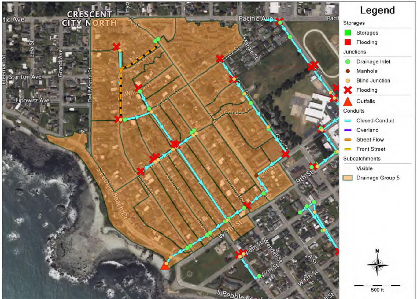
Figure 6.8 Flooding Location(s) within Drainage Group 5 for the 10-year Storm and Tidal Event
