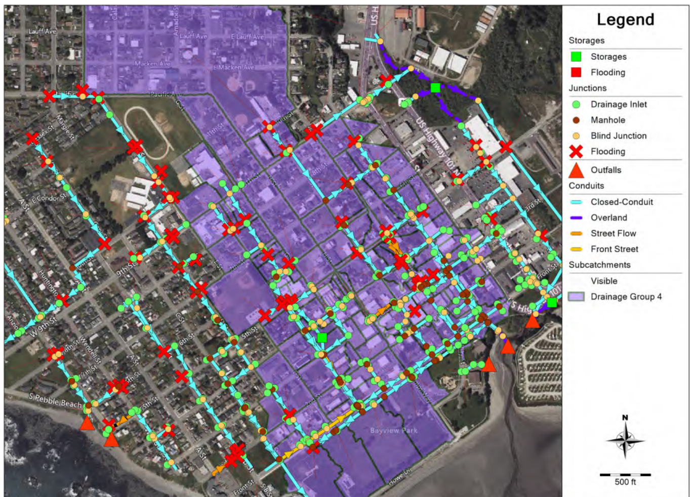
Figure 6.7 Flooding Location(s) within Drainage Group 4 for the 10-year Storm and Tidal Event
