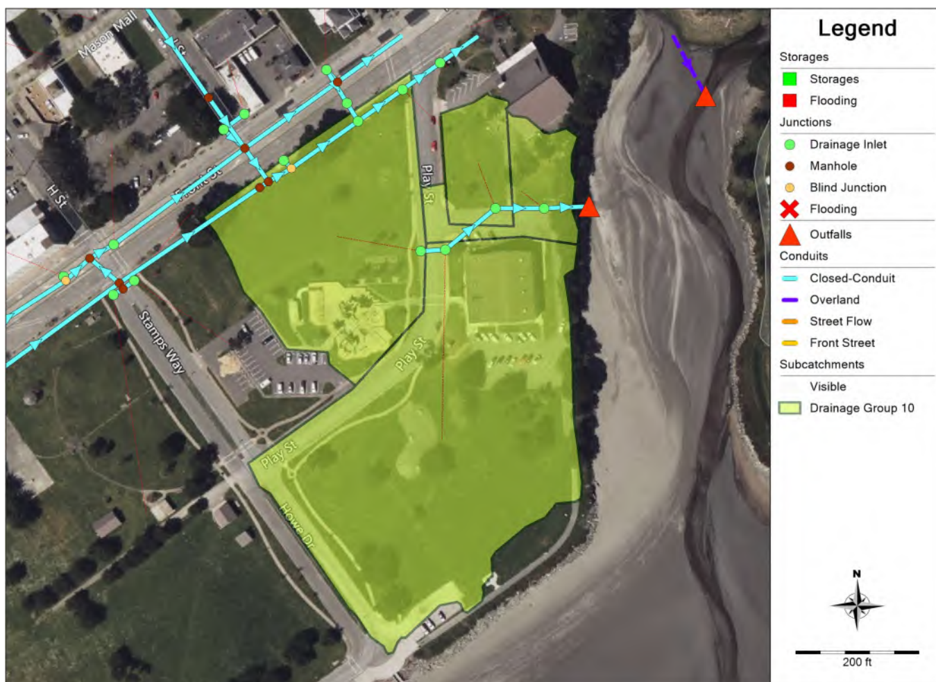
Figure 6.13 Flooding Location(s) within Drainage Group 10 for the 10-year storm and tidal event.
